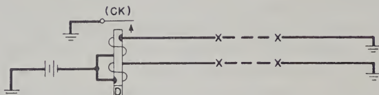
Fig. 19-21 Differential Relay Check of Two Leads
