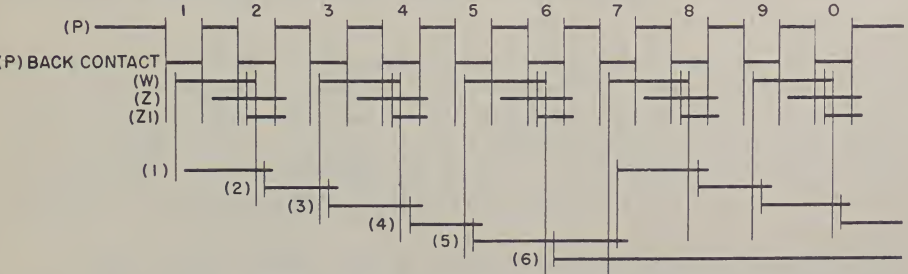
Fig. 24-5 Sequence Diagram of Counting Circuit
