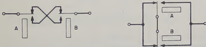
Fig. 4-33 "Only One of Two Operated" Symmetric Circuits
