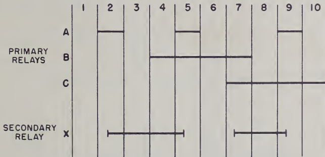
Fig. 8-8 Sequence with Two operation of a Secondary Relay
